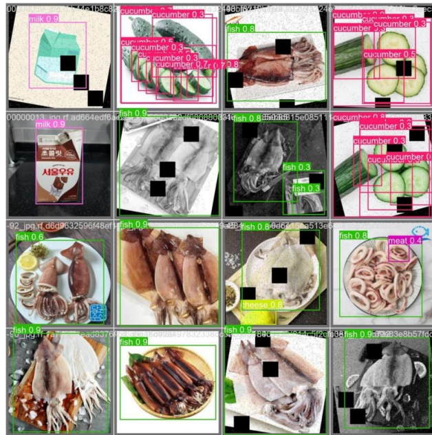
Figure 2 Example detection results on refrigerator images, including successful predictions and representative failure cases under occlusion and object overlap
